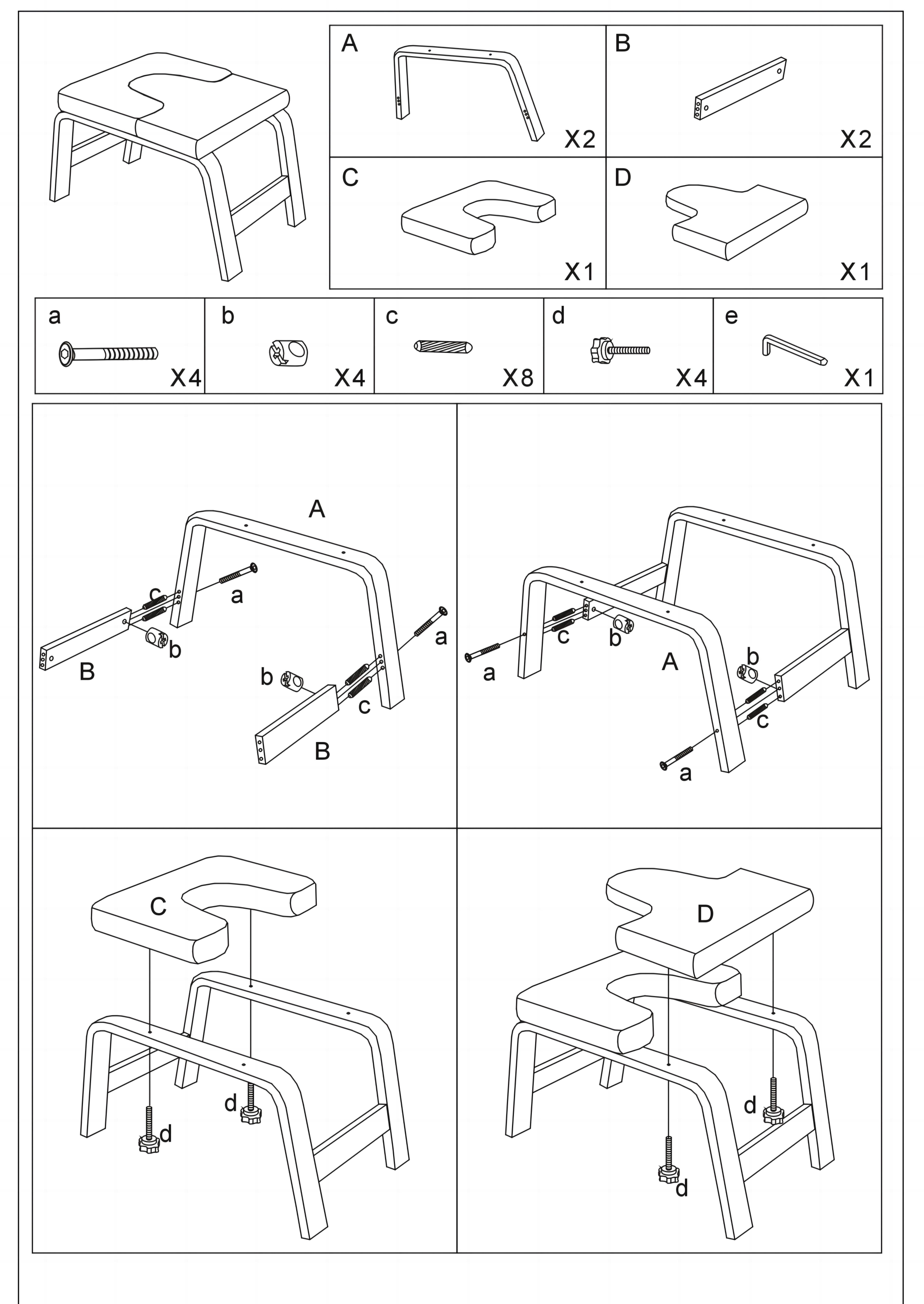
Note:When you install the "B"board, the side with the screw holes should face the inside. If you encounter other problems, you can contact us directly.
